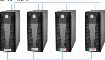
The standard version can be simply interconnected up to 4 units using the CAN-bus RJ45 cables on the rear of the SPe series UPS. The SPe series UPS uses an inverter control technology that allows to achieve N+1 scalable redundant power without the use of additional components.
